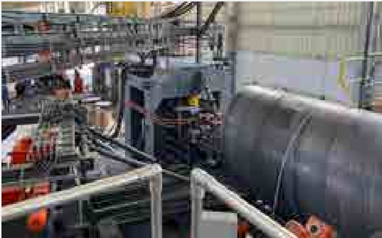
Spiral pipe mill with an adjustable diameter range from 20" (508 mm) to 120" (3,048 mm), ensuring flexible pipe production.
